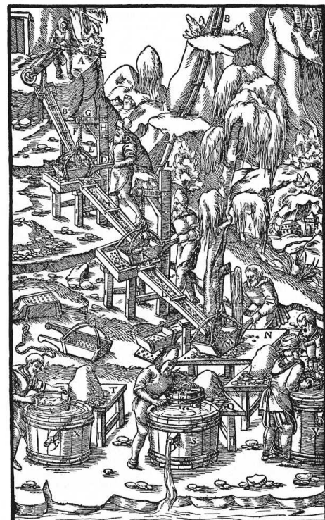
A—WORKMAN CARRYING BROKEN ROCK IN A BARROW. B—FIRST CHUTE. C—FIRST BOX. D—ITS HANDLES. E—ITS BAILS. F—ROPE. G—BEAM. H—POST. I—SECOND CHUTE. K—SECOND BOX. L—THIRD CHUTE. M—THIRD BOX. N—FIRST TABLE. O—FIRST SIEVE. P—FIRST TUB. Q—SECOND TABLE. R—SECOND SIEVE. S—SECOND TUB. T—THIRD TABLE. V—THIRD SIEVE. X—THIRD TUB. Y—PLUGS.
