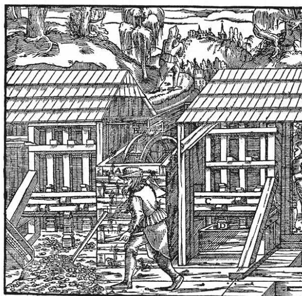
A—BOX. ALTHOUGH THE UPPER PART IS NOT OPEN, IT IS SHOWN OPEN HERE, THAT THE WHEEL MAY BE SEEN. B—WHEEL. C—CAM-SHAFT. D—STAMPS.
